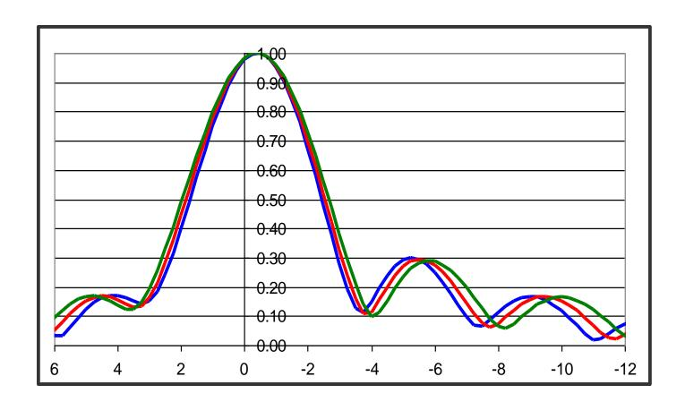
Here is the zoomed in plot of the elevation pattern we saw on page 2. The RED pattern is 360 degree, or 1 wavelength spaced at channel 25. Notice the main beam on channel 20 GREEN is slightly wider than channels 25 or 20. Which of the three elevation patterns has the highest gain ?
