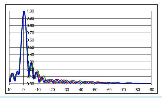
The plot above is for one of our 16 Bay half wave spaced SFN slot antennas. The RED plot is for channel 25, the GREEN is for channel 20 and the BLUE is for channel 30. With half wave and close to half wave spacing, there is very little radiation from about - 45 degrees to - 90 degrees. With little radiation at higher depression angles, the elevation gain of the main beam increases over a standard spaced array. In this model the elevation gain is 7.4% higher using the half wave spaced model.
