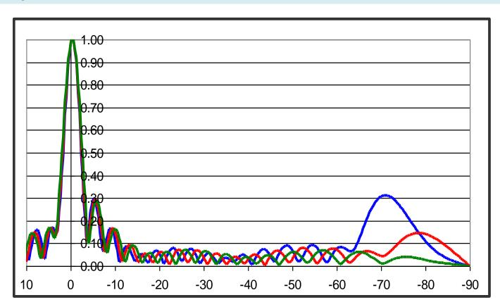
Here is the plot of the standard 16 bay antenna, with 0.5 degree of beam tilt. The RED plot is at channel 25, the GREEN plot is at channel 20, and the BLUE plot is at channel 30. Note the large lower grazing lobe that has formed at channel 30. As the spacing at channel 30 is more than 1 wavelength, the grazing lobe will get bigger. At channel 20 (GREEN), the spacing is below 1 wavelength. This will suppress the grazing lobe at -75 degrees.
